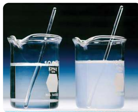
Figure (29) Sodium carbonate dissolves in water, while calcium carbonate does not dissolve in water
