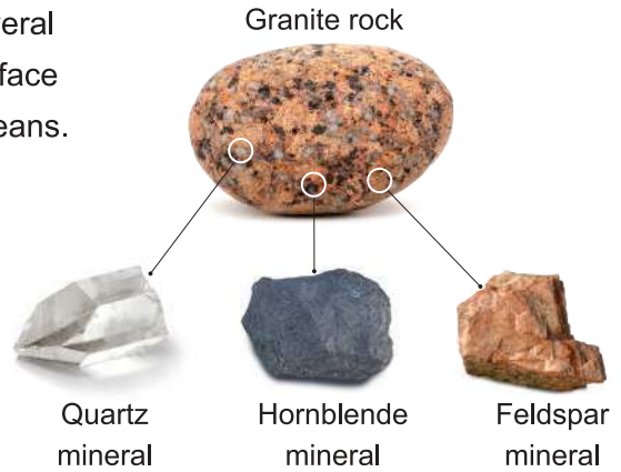
Figure (1) The minerals constituting granite rock (Names of minerals are for illustration only)
