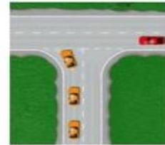
T-junction (BrE) T-intersection (AmE)
