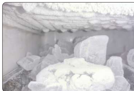
Figure (7) Water freezing in the freezer of the fridge due to heat loss
