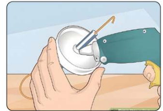
Figure (24) (6) Fix the juice straw in the bottle cap using hot glue
