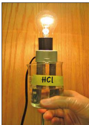
▲ Figure (16) A strong acid conducts an electrical current to a greater extent than a weak acid
